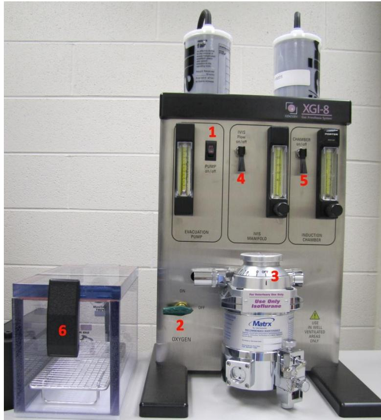
1. Weigh the F-air Canisters (located on the top of the XGI-8)
